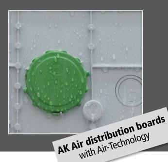
During development of the new series of distribution boards with their standard AIR ventilation element to prevent condensation, the IEC as well as the UL standards were taken into account. For that reason, materials were selected that are resistant to UV and to adverse weather conditions. Sealing systems optimised for the "Raintest' UL inspection and retaining points provided outside the sealing area on the enclosure.
